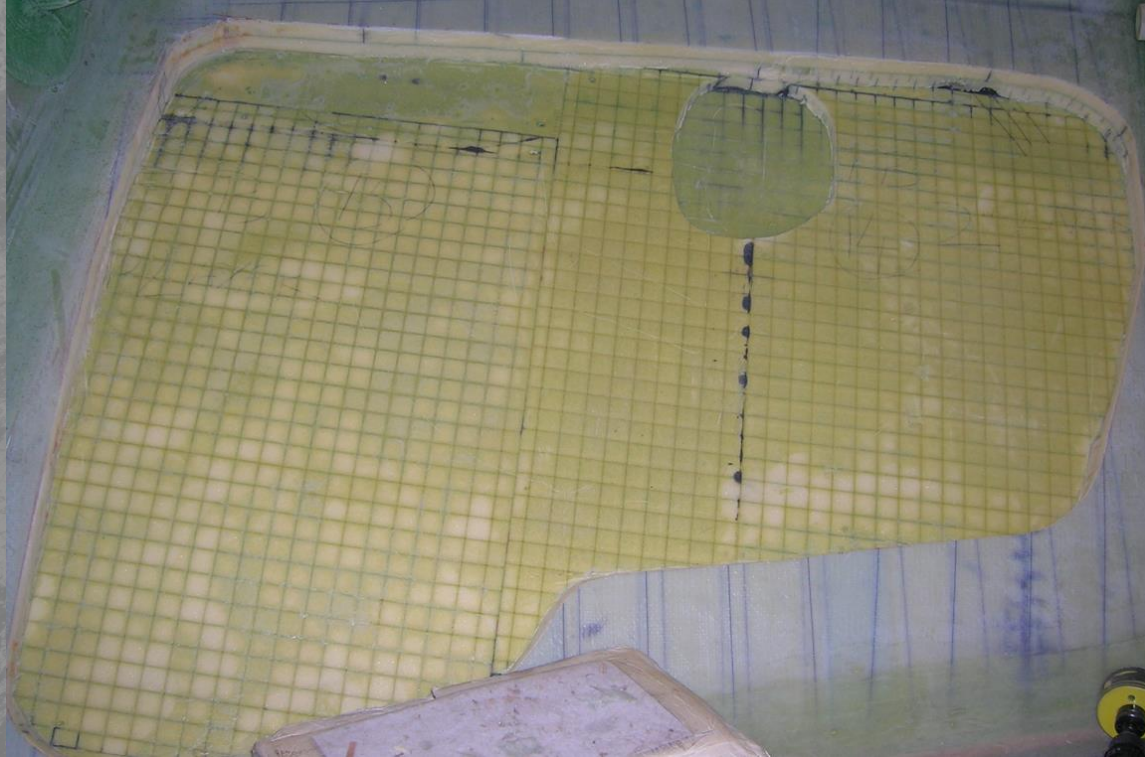
Shearography: Hull topsides – core to core disbond
